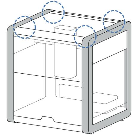
To install onto the OT-2, **slip the key corners on the left hand side of the adaptor** bracket under the sheet metal of the robot as shown below.
